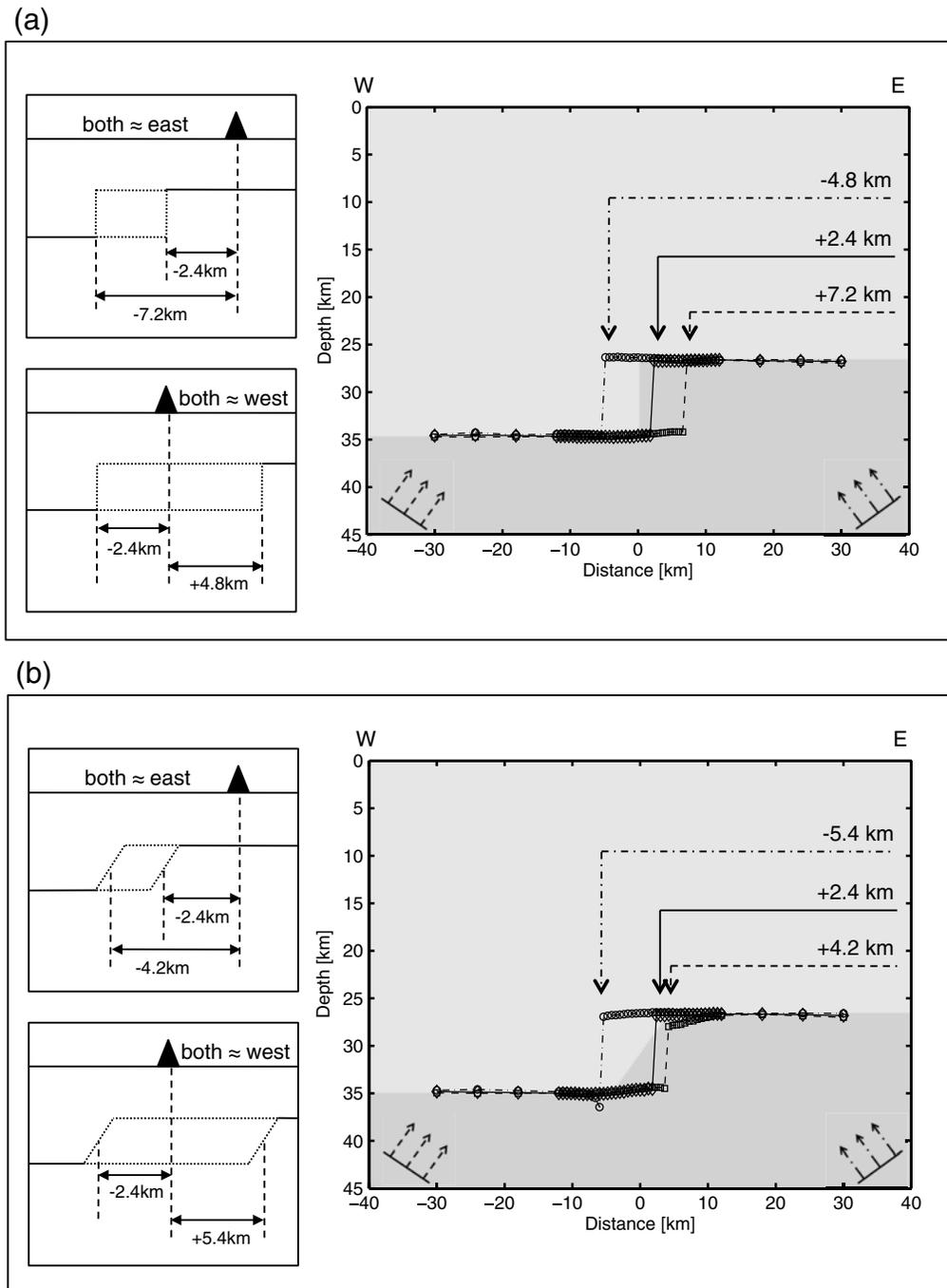
**Figure 12.** Lateral location ranges of an 8 km Moho offset from single-station RF analysis (noise free, (a) step model, (b) ramp model). See ⑤ Figures S11 and S12 for the location ranges for the models with added noise.
