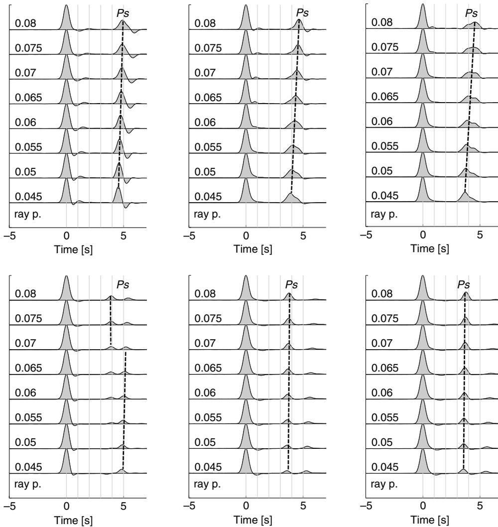
**Figure 11.** RFs for the Moho ramp model. The top row shows RFs at stations (left)  $-7.8$ , (center)  $0.0$ , and (right)  $+3.0$  km, with seismic waves traveling from the deep Moho side. The bottom row shows RFs at stations (left)  $-7.8$ , (center)  $0.0$ , and (right)  $+3.0$  km, with seismic waves traveling from the shallow Moho side. Peak  $P_S$  arrivals are outlined by dashed lines. The numbers on the left of the RFs list the ray parameters.
