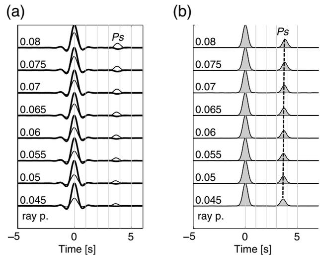
**Figure 6.** (a) Synthetic seismograms at station 51 calculated in the reference model. The vertical components are shown in thick black lines, and the radial components are shown in thin gray lines. (b) RFs estimated from the synthetic seismograms. The ray parameters are listed at the left of their waveforms. Peak  $P_S$  arrivals are outlined by the dashed line. The numbers on the left of the seismograms and RFs list the ray parameters.
