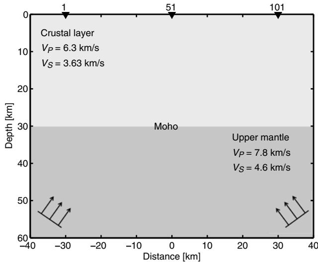
**Figure 5.** Reference layer-over-half-space model with a flat Moho. Distance 0 km is defined at the center of the model along the radial direction; 101 receivers are located on the surface between  $-30$  and  $+30$  km. The three triangles depict locations of receivers at  $-30$ ,  $0$ , and  $+30$  km, as stations 1, 51, and 101, respectively. Arrows show the directions of the incident planar  $P$  waves.
