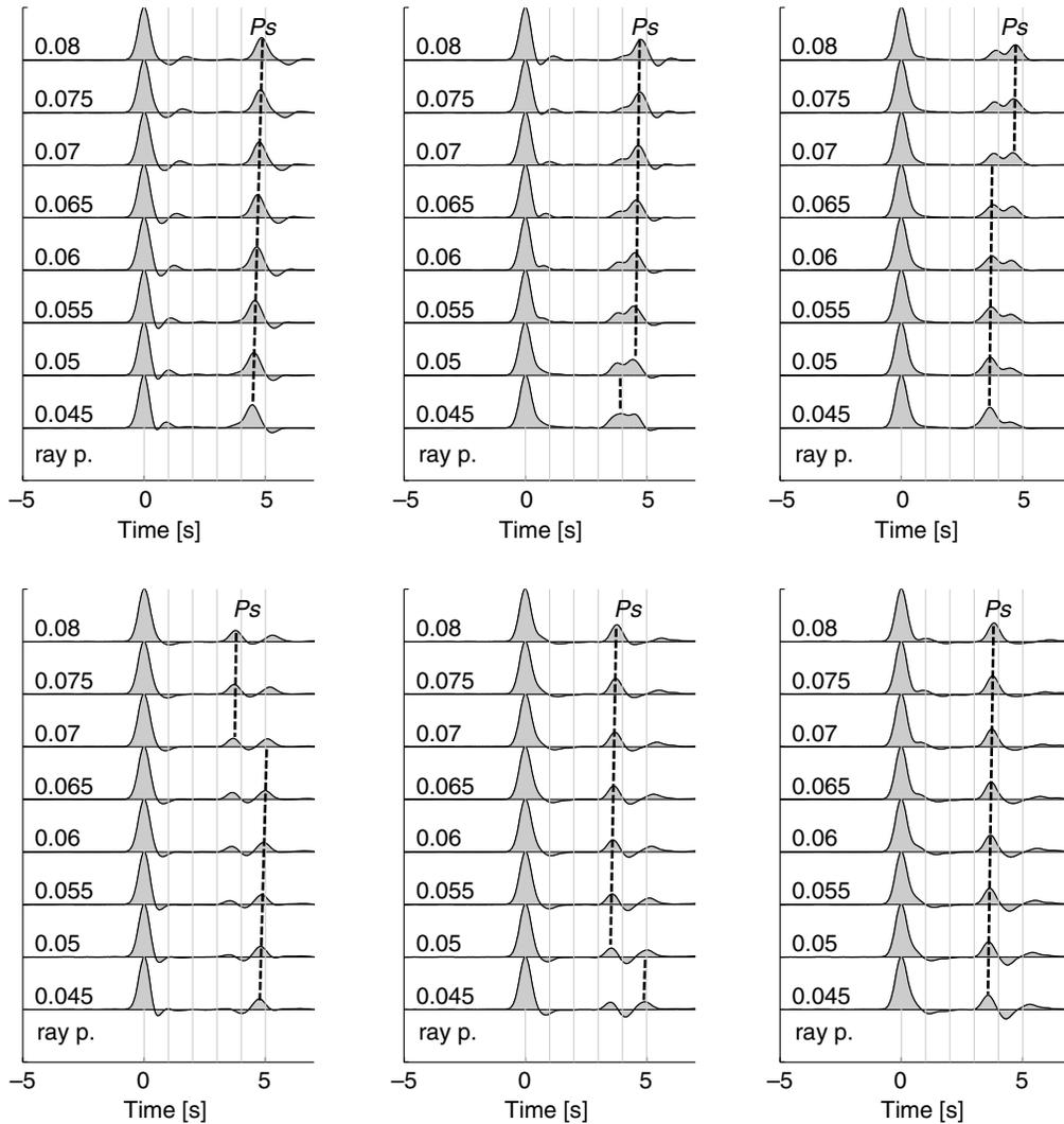
**Figure 9.** RFs for the Moho step model in Figure 8a (step model). The top row shows RFs at stations (left)  $-6.6$ , (center)  $-1.2$ , and (right)  $+4.2$  km, with seismic waves traveling from the deep Moho side. The bottom row shows RFs at stations (left)  $-6.6$  km, (center)  $-1.2$  km, and (right)  $+4.2$  km, with seismic waves traveling from the shallow Moho side. Peak  $P_S$  arrivals are outlined by dashed lines. The numbers on the left of the RFs list the ray parameters.
