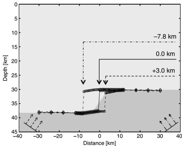
**Figure 10.** Ramp model and estimated Moho depth from the ZK2000 method for a Moho ramp between  $-3.9$  and  $+3.9$  km. The locations of stations  $-7.8$ ,  $0.0$ , and  $+3.0$  km depict the horizontal locations of the abrupt change in Moho for the three source scenarios (from the deep side, the shallow side, and both sides). See Figure 8 for the notation of the lines and points.
