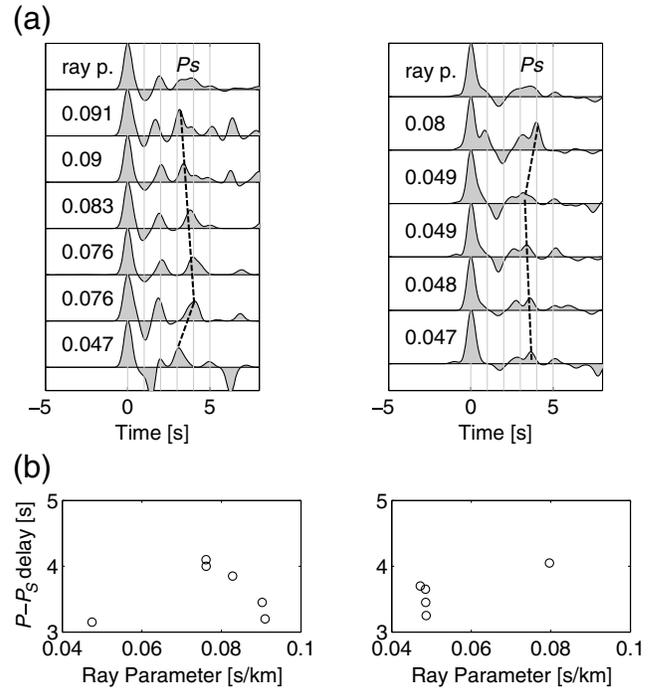
**Figure 3.** (a) Receiver functions (RFs) at station LKR as a function of ray parameters (ray p.) for sources incident from (left) the west and (right) the east. Peak  $P_S$  arrivals are outlined by dashed lines. The numbers on the left of the RFs list the ray parameters. The uppermost RFs are generated from a stack of all RFs shown below. (b)  $P$ – $P_S$  delay times for sources incident from (left) the west and (right) the east.
