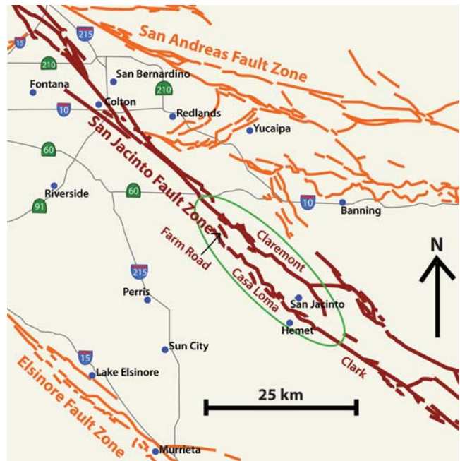
Figure 2. Close up of the northern SJF zone with geometry based on the U.S. Geological Survey (USGS) Quaternary Faults Database (see Data and Resources ). The Claremont–Casa Loma stepover is circled in green. The Claremont strand is the more northeasterly of the two; the Casa Loma is to the southwest. The small fault within the northern end of the stepover is the Farm Road strand.
